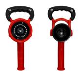
With a hard anodised aluminium body and ABS handle with a rubber bumper, the Vigil 230 selectable fire nozzle has a lightweight and robust design that's perfect for demanding environments. The stainless–steel spinning teeth create different fog patterns, while the laser engraved settings on the body ensure you can see the various settings available.
