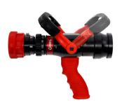
Manufactured for Vigil Products in accordance with BSEN-15182, the selectable fire nozzle has a maximum flow of 230 litres per minute with a 6 bar working pressure. It comes complete with an integral 2  $\frac{1}{2}$ " instantaneous alloy male inlet (BS 336) for UK fixings.
