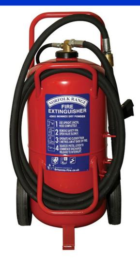
Monnex is based Potassium on bicarbonate Urea complex. extinguishing powder interferes with the chemical reactions that take place in the combustion zone, thus the flame ceases to exist and the fire is extinguished. In the combustion zone Monnex powder explodes breaking into smaller particles which dramatically increases the surface area of the powder and thus the speed and effectiveness of this product.
