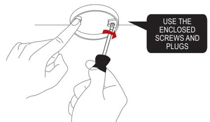
Once the mounting base is installed, attach the alarm by twisting clockwise until it clicks. If the battery is either missing or inserted incorrectly, or the switch is in 'Learn Mode', the smoke alarm will not be able to click into the mounting base.
