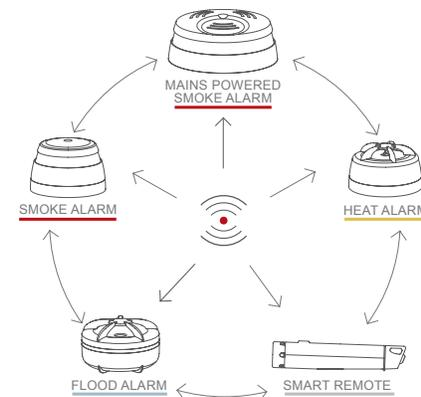
All CAVIUS interconnected alarms within the **WIRELESS** ALARM FAMILY can be added to the system as they run on the same frequency and use the same data protocol. This means that the wireless system can consist of a combination of smoke, heat, flood etc.
