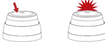
When all alarms flash the red LED, they are connected and can be switched out of 'Learn Mode' and installed.
