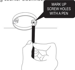
Use the mounting base ring to mark the screw holes on the ceiling or the wall.
