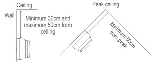
With a minimum of one smoke alarm per floor and a maximum distance between smoke alarms of 10 meters.
