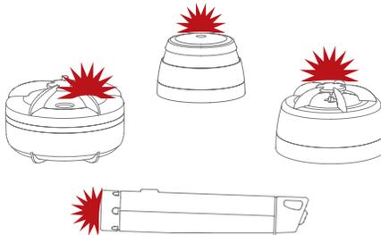
**6.** When all alarms flash the red LED, they are connected and can be switched out of "Learn mode" and installed.
